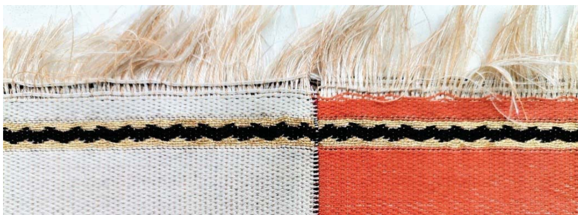
FIGURE 9. Connecting different colored wefts in the middle of the belt with bass threads.
